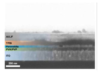
Fig. S15 Cross-section SEM image of the PeLEDs.
